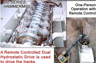
The operator of the loader or excavator can stay safely inside the cab while moving the HogZilla Grinder to different locations allowing one-person operation.
