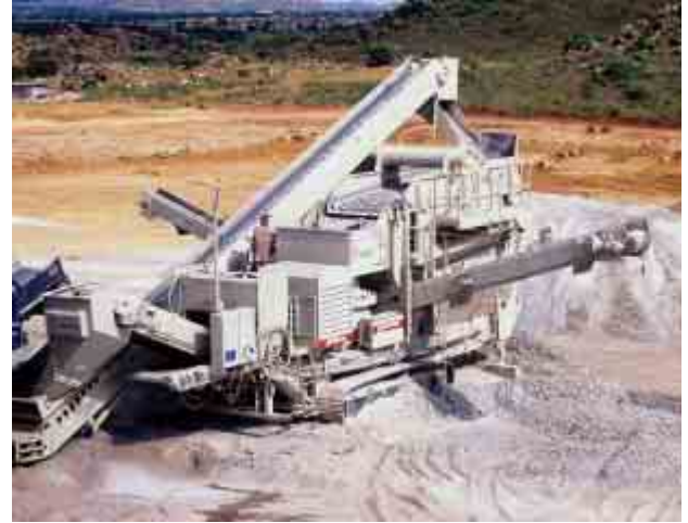
Lokotrack LT1100 cone plant.
