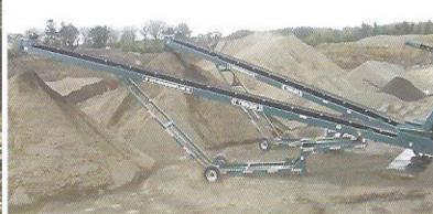
The Mk II is a cost efficient mobile scalping and screening unit used extensively to screen material such as sand and gravel, coal and topsoil.
