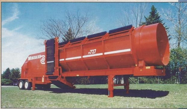
The Morbark PT727 is purposely designed to be **heavy in strategic areas** in order to effortlessly withstand the rough, tough treatment of compost, yard waste, wood grinding, C & D and land clearing projects. The heavy duty 27' long x 7' diameter trommel tube is constructed of 3/8" thick steel plate which holds its shape even when processing bulky, heavy material. The trommel is supported by four 8"
