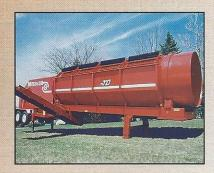
Once the proper angle is set, support legs are pinned and pressure on the hydraulic cylinders can be relieved. This adds life to the cylinders and stability to the machine.
