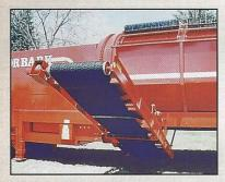
A unique straight through, unrestricted throat opening from hopper to trommel allows the PT727 to accept bulky material without jamming or plugging.
