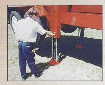
The fines stacking conveyor unfolds for operation at the touch of a lever. After only about 10 minutes set-up time, the PT727 is ready to run.
