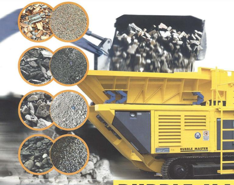
The RM 80 processes asphalt, concrete, rock and general construction/demolition debris up to 150 t/h. Feed sizes up to 2'-3 1/2" are turned into a high-quality cubic grain end product in a fraction of 0 - 1 1/8" to 0 - 2 3/4" (ideal for further processing).
