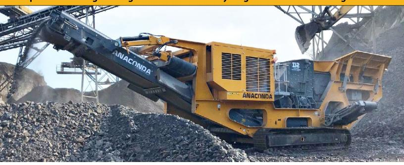
The Anaconda Range of Mobile Tracked Impact Crushers are designed specifically to suit applications where the toughest demands of primary crushing are of imperative importance with their immense power, reliability and productivity.
