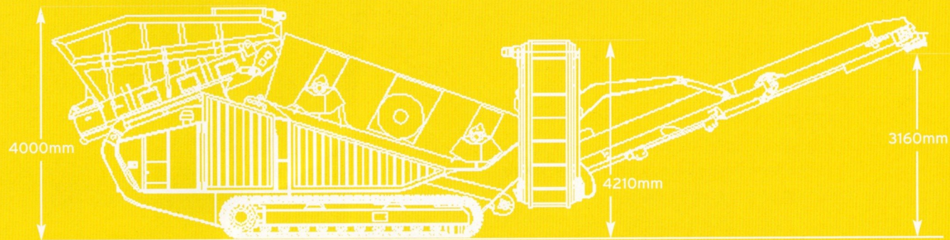
Viper Discovery side elevation - in working position
