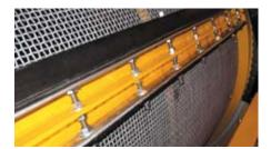
Our exclusive tensioned-screen panels — manufactured by Wildcat, and available on all trommel screen line models — add strength to the panel and accommodates the installation of smaller-diameter wire when the material allows. This increases production capacity and minimizes sticking, enabling wetter material to be processed.
