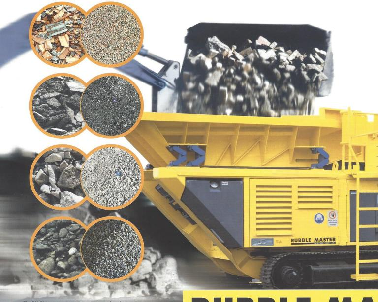
The RM 80 processes asphalt, concrete, rock and general construction/demolition debris up to 150 t/h. Feed sizes up to 700 mm are turned into a high-quality cubic grain end product in a fraction of 0 - 30 mm to 0 - 70 mm (ideal for further processing).
