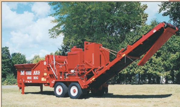
The compact Model 3600 Wood Hog gives contractors, municipalities and wood waste processors another important option in wood waste recycling equipment. With power options ranging from 325-540 HP, along with Morbark's customary, heavy-duty construction, the 3600 has the muscle and size to process a
