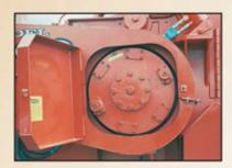
A hinged door allows quick and easy access for changing hammers, tips and grates.
