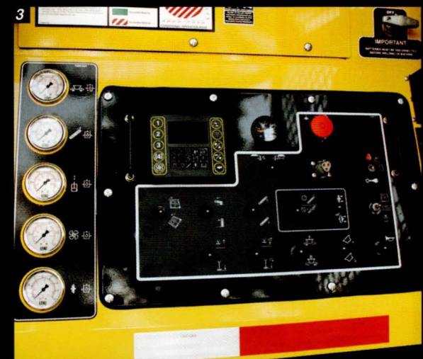
3: Control Panel. Providing a digital readout for the microprocessor and the CAT engine, the control panel gives the operator real-time performance information and full instrumentation and fault code displays for monitoring systems and troubleshooting.
