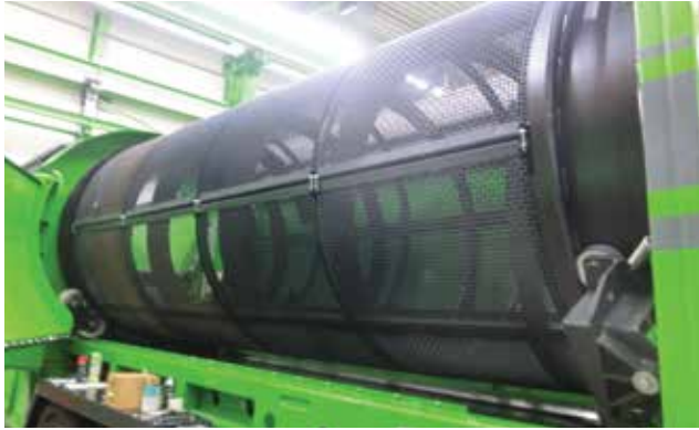
Full side door for easy drum exchange
