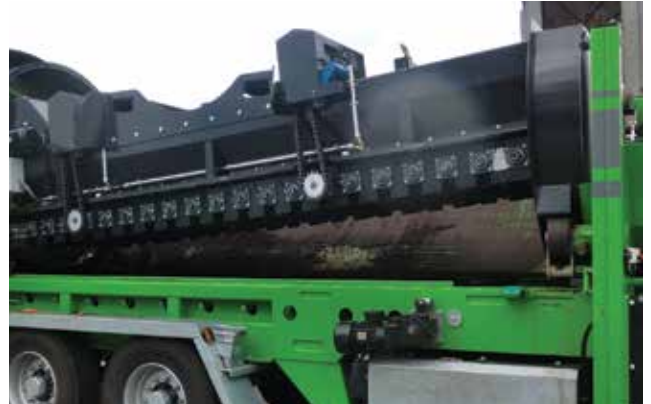
Star screen insert. 1 piece fines belt prevent spillage at transfer point
