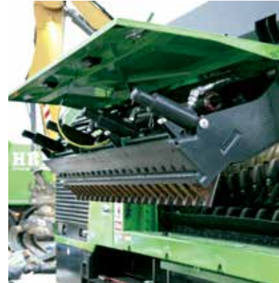
Hydraulic fold up counter comb
