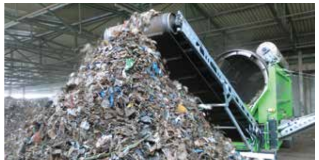
Star screen insert. 1 piece fines belt prevent spillage at transfer point
