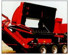
The tub and table tilt 90 degrees for emptying and easy servicing of the hammermill.
