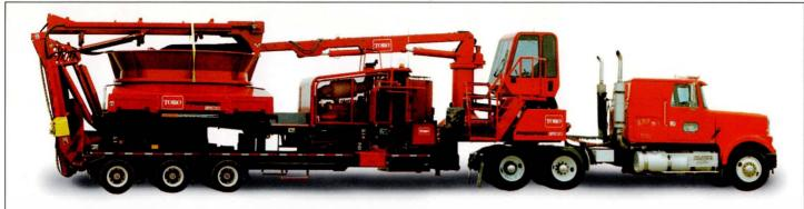
The ProGrind 5100 conveyor and grapple fold for transport, allowing quick and easy movement of the grinder from job site to job site.
