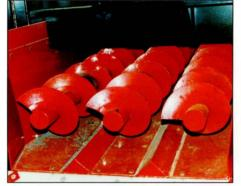
Triple 12" discharge augers provide the needed movement of material from mill area to stacking conveyor for this high production unit.
