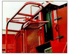
A protective canopy provides safety for operators by guarding against falling objects.
