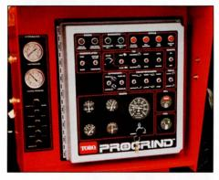
Conveniently located and easy to understand, the control panel provides maximum operational information to make grinding efficient, simple and safe.
