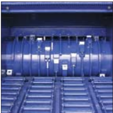
The heavy duty rotor is continuously fed by a chain conveyor.
