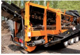
The two-deck star screen mechanism of the SM 1200 delivers precise separation at extremely high rates of output.
