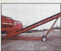
Equipped with a road-legal fifth-wheel towing arrangement, the Model PT837 is completely portable, with a set-up time of approximately 10 minutes.
