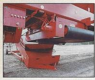
The portable fines stacking conveyor may be quickly positioned on either side of the trommel without having to move the machine.
