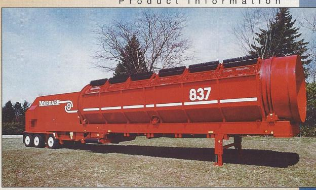
As the world's largest portable trommel screen, the Morbark Model PT837 packs not only the size, but the horsepower, hydraulic muscle, torque and innovative design features required to tackle the most demanding applications. The PT837 is built critically heavy in strategic areas, from the main frame rails and tube to the hydraulic system—all are designed to carry tremendous loads without wavering. Material flows from the 12 yard
