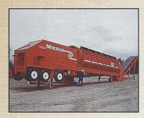
The throat opening, a unique straight through design from hopper to trommel, is completely unrestricted, allowing the unit to accept very bulky material with ease.
