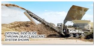
One loader or excavator operator can feed the HogZilla, controlling it by remote control and the optional 60° radial stacking elevator enables longer production runs.
