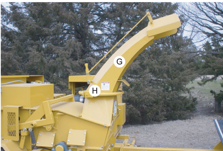
Forward directing discharge for easy and accurate positioning of material
