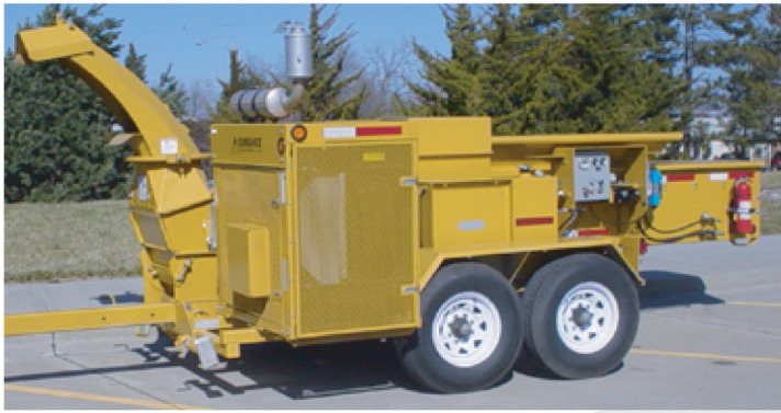
Engine and Control side of Grinder
