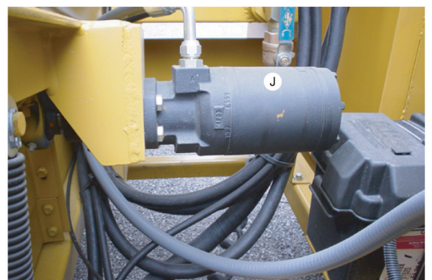
Heavy Duty Hydraulic Motor Turns Feed Roll
