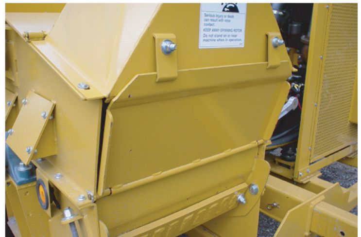
Hammer access panel in operating position and exclusive grinding fingers where final particle reduction takes place
