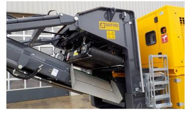
Barford 750J - 700 x 500 (28" x 20") Tracked Dual Power Jaw Crusher, Reversible Jaw, 88Kva Diesel Generator/Mains Plug In, Vibrating Grizzly Feeder, Hardox Lined Hopper, Feed Sensor, Auto Feed System, Radio Remote for Feeder Stop/Start, Weight 19,000kg / 40,000 lbs, Fits in a 40Ft container
