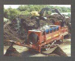
Feeder automatically meters material into screening drum thereby maintaining the efficiency of the screening operation.
