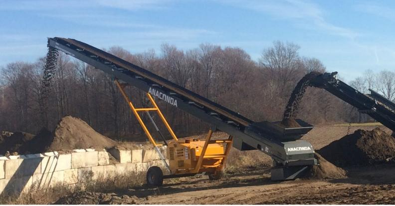
The Anaconda ST Range of Mobile Wheeled Conveyors are designed for the Material Handling Sector and aim to reduce production time and save stockpiling costs.
