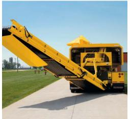
Radial stacking conveyor. The rear uploading conveyor oscillates 60 degrees allowing the operator to change placement of the processed material without moving the machine. The conveyor may be equipped with an optional magnetic head pulley to help remove steel metallic materials, resulting in a more useful end product.
