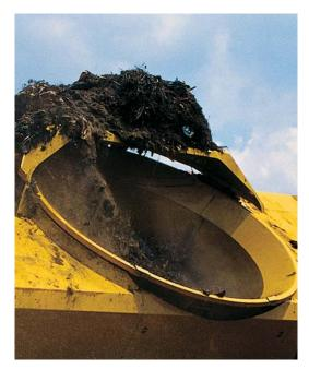
To allow large loads, the TG9000 unit features the largest inside tub diameter in the industry. It has an 11' (3.4 m) inside diameter and a folding 13.6' (4.1 m) flare opening.
