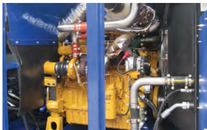
LRC - CATERPILLAR C9 310Kw (420HP)
