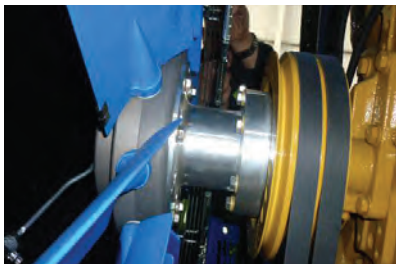
Reversible Fan - recommended for dusty applications
