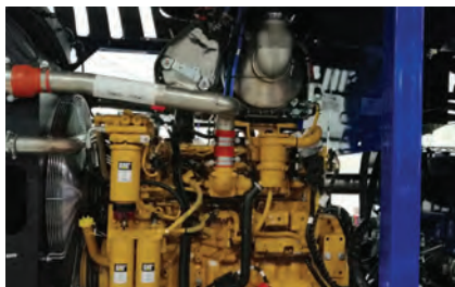
Tier 4 Final / Stage 5 - CATERPILLAR C9.3B 310Kw (420HP)
