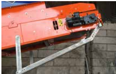
Magnet Head Drum and Chute (Mid-Weight) - Ferrous metal extraction
