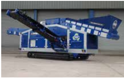
Tracked Mounted - Fully tracked for on-site manoeuvrability
