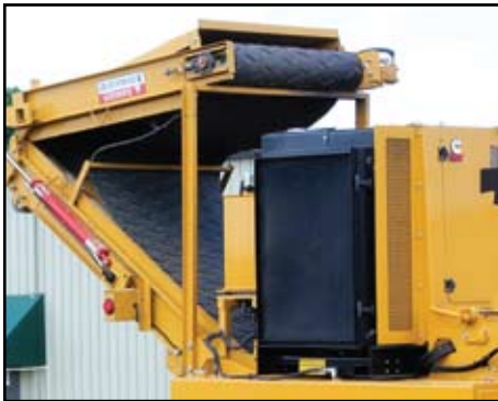
Folding extended discharge conveyor With magnetic head pulley
