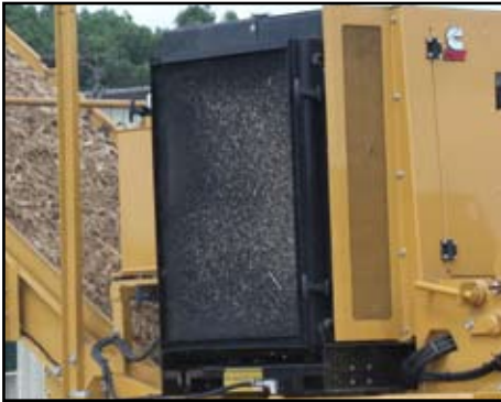
Oversized radiator with reversing fan and Removable debris screen
