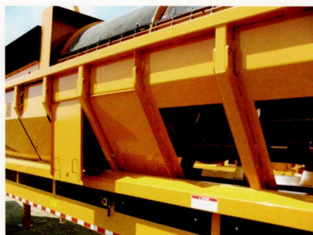
Removable panels along drum for cleaning.
