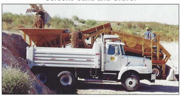
**Conveyors Can Load Directly Into Truck**
