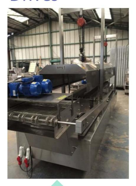
Our fryers have separate variable speed drives for top and bottom belts allowing more control. This also allows for floating product to be fried then the bottom belt speed increased to remove product quickly, giving less product binding
