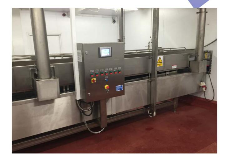
The oil circulation pump fitted to the fryers ensure a constant even temperature over the full length of the fryers.
