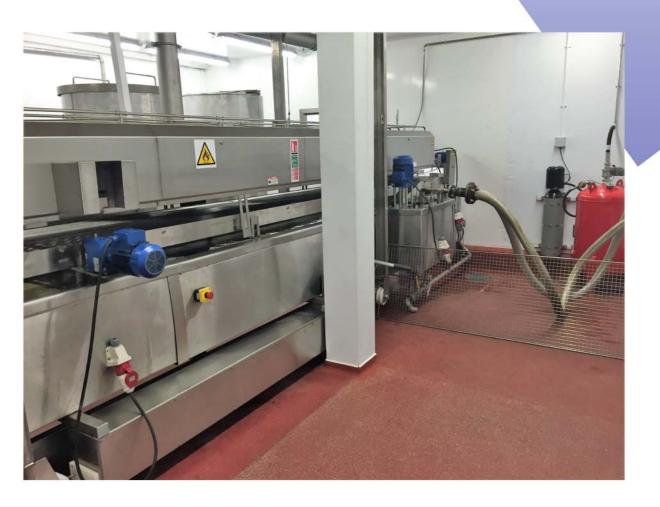
The combination of adjustable oil flow and an adjustable belt height enables our fryers to maintain excellent product orientation which prevents two products from sticking together. It also delivers consistent product quality even with very high belt loads, as the product remains evenly distributed and are not pushed around by the oil flow. This approach ensures that the oil temperature remains virtually constant along the full length of
