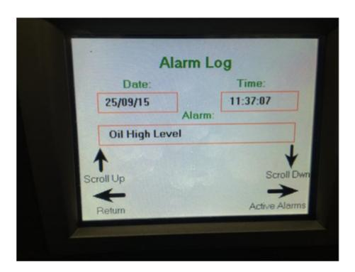
A full range of alarm systems are standard on PLC controlled machines.
