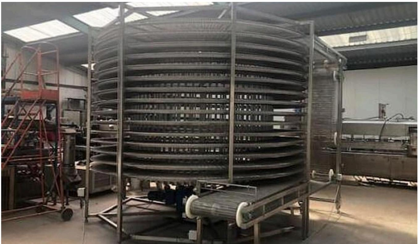
**Spiral coolers can be made with an open drum as in the picture this enables fans to blow the heat away much more efficiently, used a lot for bread and bakery products.**
