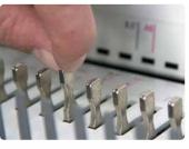
QSA (Quick Size Adjustment) technology allows the punching pins to be cancelled and the paper formats to be changed quickly and easily.
