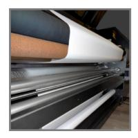
• For stretchable fabrics like Lycra, spandex and other sports textiles, the Eos uses a cork-covered cylinder to spread and hold the fabric in place, maintaining perfect, precise print quality.
