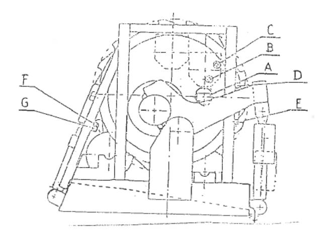
Ahlstrom Drum Press (Model DP-2200) Installed in 1988. Used for about two years. Been unused since. Nominal capacity of the Press is 2120 cubic feet per hour of loose un-pressed material.
