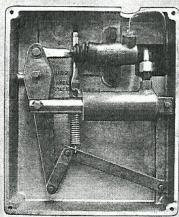
Optional Control permits fine adjustment of the web alignment from remote locations. This is particularly valuable at the double backer where it allows operator to adjust position of the liner stands while observing combining of single face and liner.
