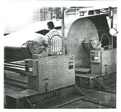
Roll Stand in running position with splicing operation having been completed. Note minimum core waste and convenient access to web from floor or splicing platform provided on Stand. Both operator's control and splicing platforms are of raised safety tread design.
