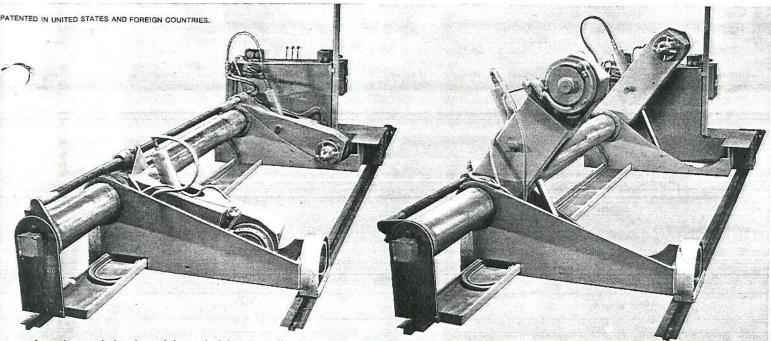
Arms lowered showing minimum height above floor, permitting loading and unloading of butt rolls as small as 18-inch diameter. Precision alignment of arms and chucks is maintained by massive backbone tube. As roll enters Stand it is automatically squared into parallel position by contacting tube.
