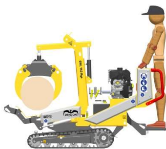
Figure 11: Log Grab Operation
