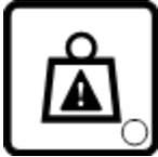
Light flashing indicates the platform is overloaded. The engine will stop and no functions will operate.
