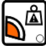
**S-60 HF, S-65 HF:** The range of motion light is on when the platform load exceeds 272 kg.
