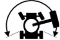
To drive, hold the drive enable switch to either side and slowly move the drive control handle off center.
