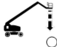
Machine On Incline indicator light is on: The light is on and the tilt alarm sounds when the machine exceeds the tilt sensor activation settings. Follow the appropriate procedure below and move the machine to a firm, level surface.
