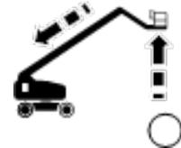
Lower Boom indicator light flashing: Lower the boom until the indicator light is off.
